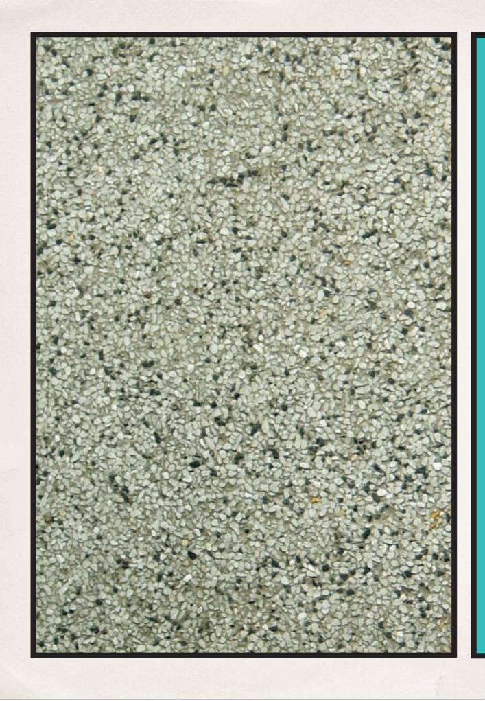
Made by mixing sand-size fne colored aggregate and cement.
